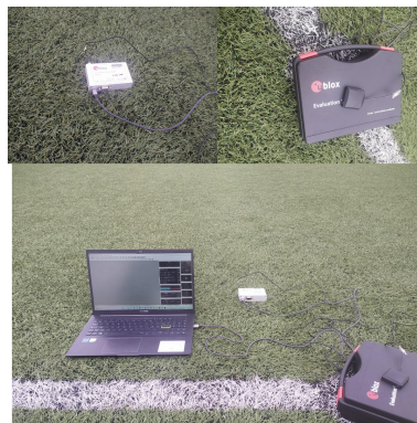
Figure 2.1: Data collection in open field-receiver, antenna and laptop with u-center
